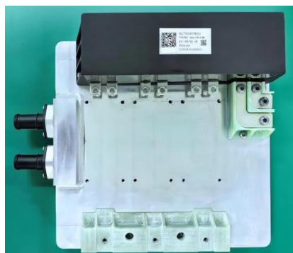
Figure 7: Common ED3 module heatsink
